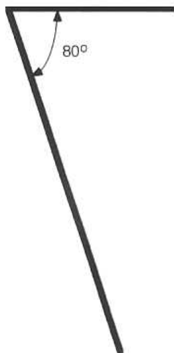
Figure 6A. Quantitative analysis of the cutting edge. Typical sharp edge with an edge angle of 80^\circ .
